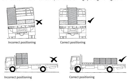
The diagrams above show examples of the incorrect and correct way of loading a heavy vehicle.
